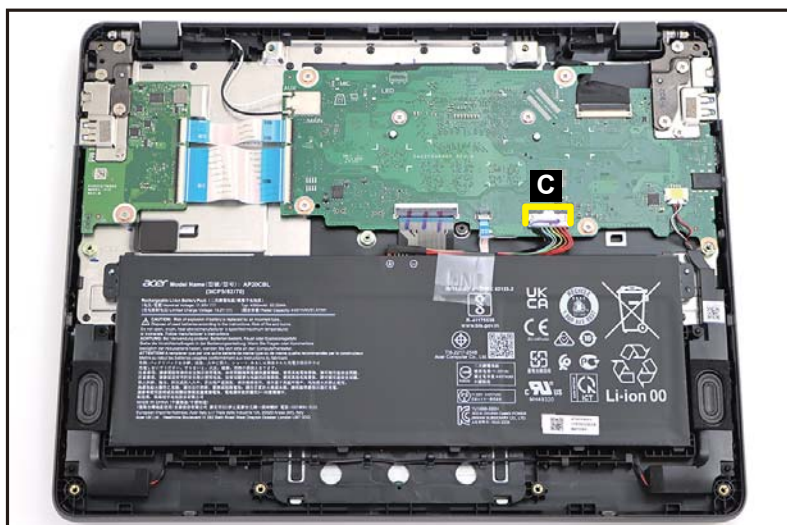
Figure 1-7. Battery Pack Removal
